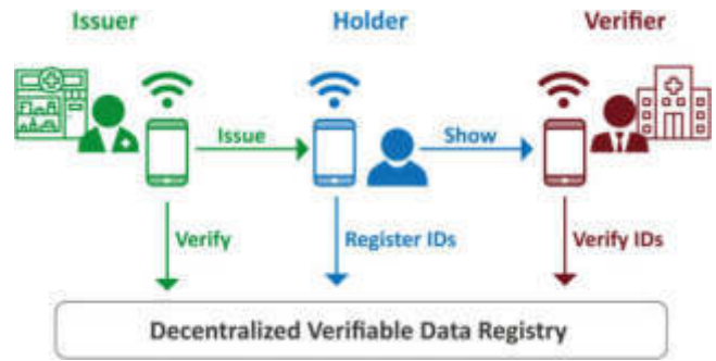
Fig. 1. Main roles and workflow in W3C Verifiable Credentials [12], adapted for our COVID-19 Antibody Testing use case.
